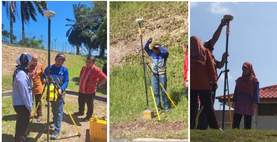
Figure 4: GNSS observations being carried out by the project team
