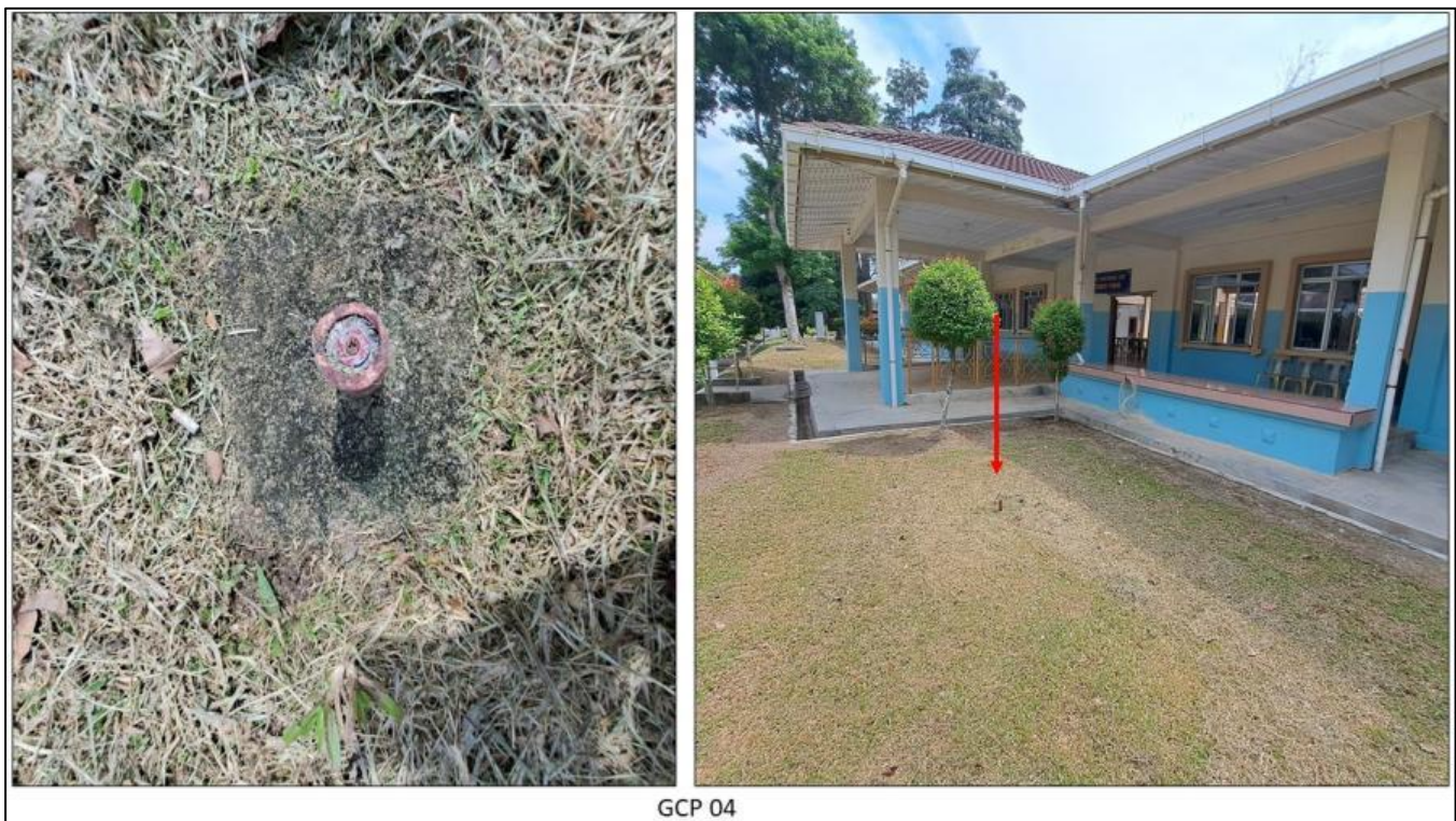
Figure 9: Position of Ground Control Point 4 (CP04) next to the PMM Dormitory Cafeteria.
