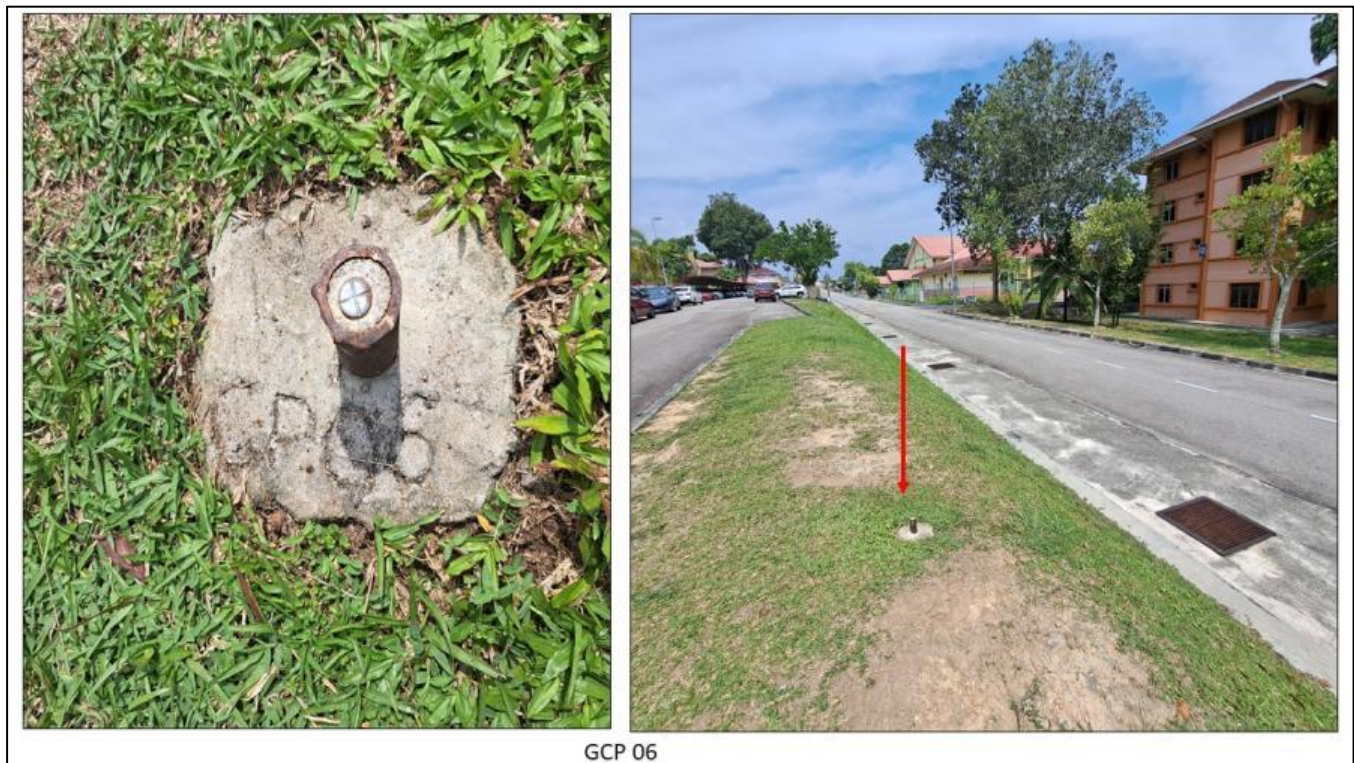
Figure 11: Position of Control Point 6 (CP06) next to the Department of Electrical Engineering (JKE) building
