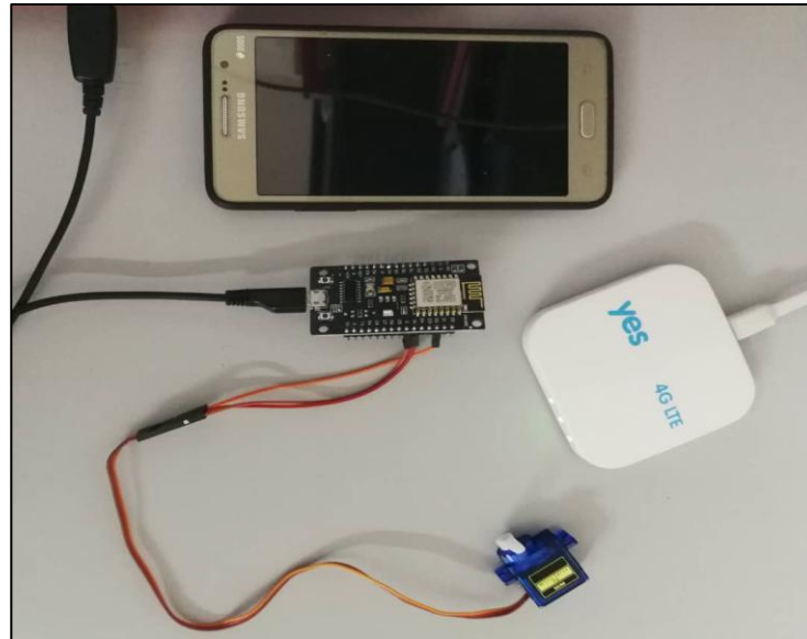
Figure 9: Setup for range testing and response time to lock and unlock the door using the website
