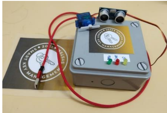
Figure 6: An Affordable Smart Key Monitoring System with IoT
