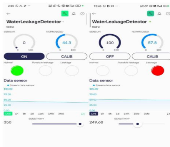
Figure 5.0 : Green Indicator ( No Leakage ) & Red Indicator ( Leakage )
