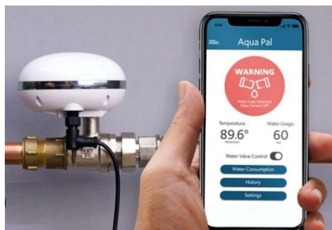
Rajah 1 : Sistem kawalan Smart Water Meter
