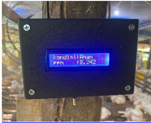
Figure 7: IoT-based air quality monitoring tool in chicken coops
