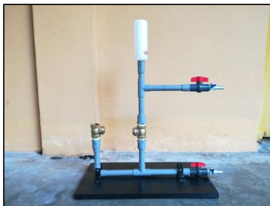
Rajah 6: Free Energy Ram Pump (FERP)
