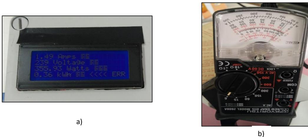
Figure 8: Measuring the current with E-MON with hair dryer a) LCD displaying the value of current & Voltage draw by hairdryer b) Clamp Meter reading on the actual current by hair dryer.
