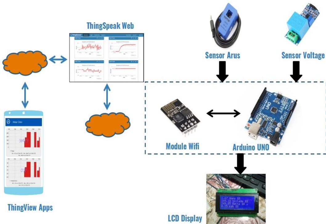
**Figure 1:** Energy Meter (E-MON) With IoT Monitoring Model
