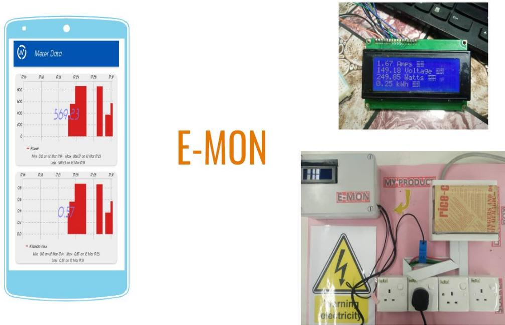
Figure 7: Final design of Energy Meter (E-MON) With IoT Monitoring
