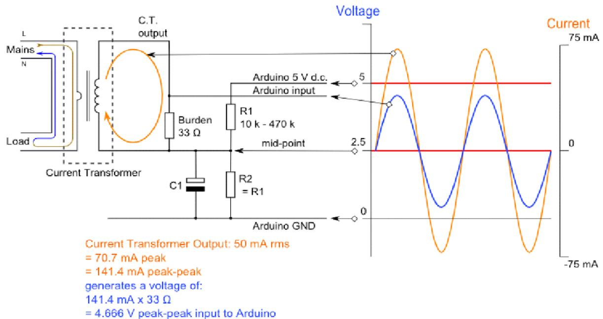
Figure 4: Calculating a suitable burden resistor for 5V input Arduino
