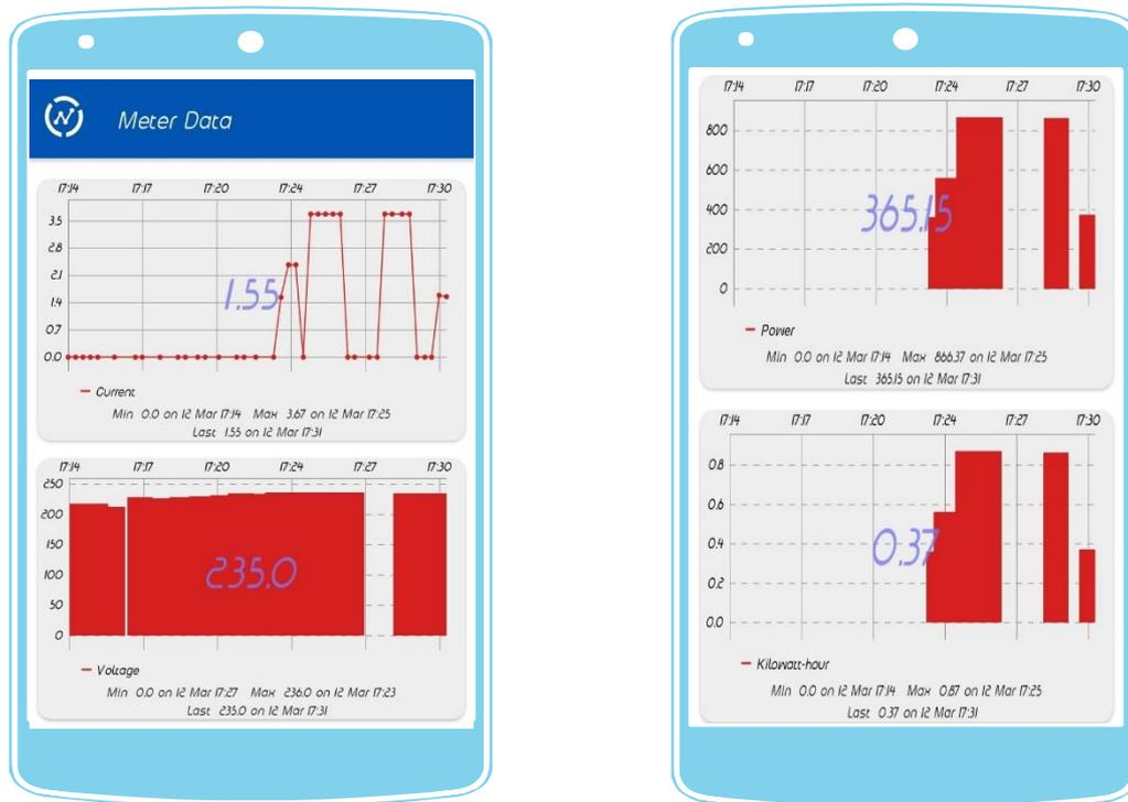
Figure 9: Energy consumption by Hair Dryer monitor via smartphone
