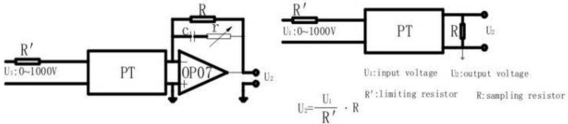
Figure 2: Wiring diagram of ZMPT101B
