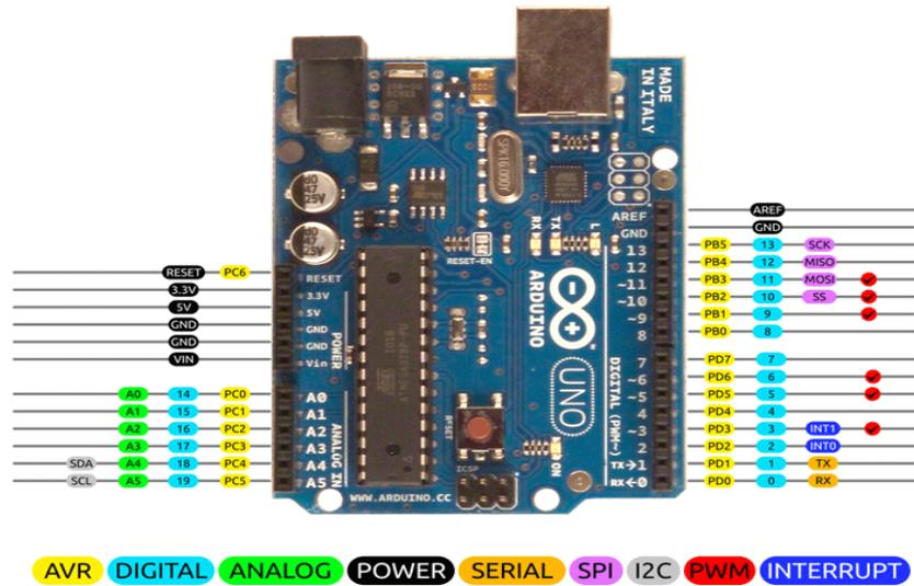
Figure 5: Pin Diagram of Arduino UNO
