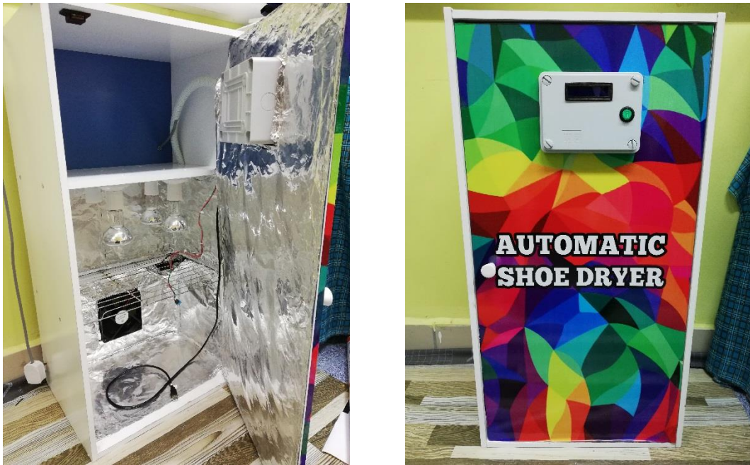
Figure 4.2 Project Design and Installation of Automatic Shoe Dryer
